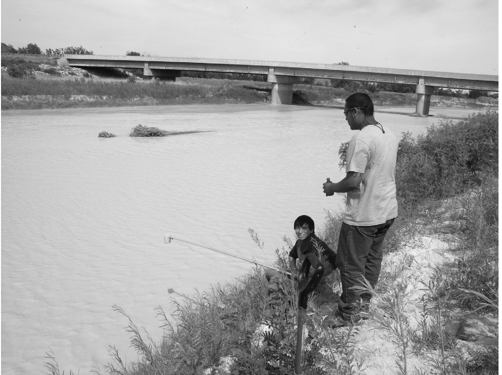
Armando Hernandez and Daniel Johns, PEEC interns from South Dakota State University, in 2012 collecting water samples from the White River on Pine Ridge Reservation in South Dakota. Samples were tested for heavy metals concentrations including As, Ba, Pb, Se, and U. Uranium is of particular interest to the community because of uranium extraction mines in the locale. (Photo credit: Joanita Kant)
