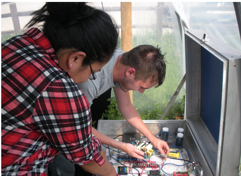
Genevieve Sandoval Bull Head and Zach Buechler, South Dakota PEEC students, assembling the climate control system for a sustainable greenhouse on the Pine Ridge Reservation. (Photo credit: J.F. Sawyer)
