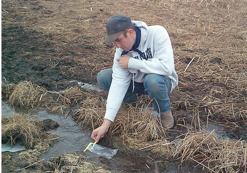
Bart Krautschun, Extension educator, takes water samples from a pasture stream. His Butte County Extension office can perform tests for total dissolved solids for ranchers concerned about water quality.
