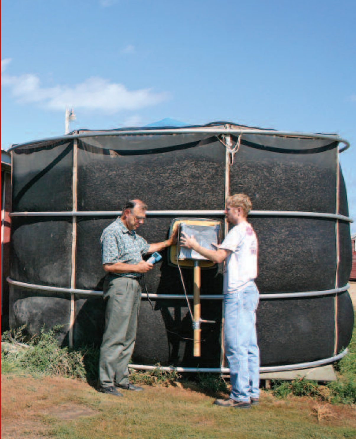
Dick Nicolai, SDSU Extension engineer, and Ryan Lefers, engineering graduate student, built a working composite vertical biofilter. This one is larger than a farm model because it is actually six different versions of a vertical biofilter; the best version will be selected for continued testing.
