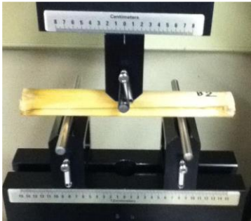
Figure 16. Three-point loading apparatus
