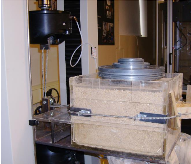
Figure 18. Experimental setup of bulk shearing test
