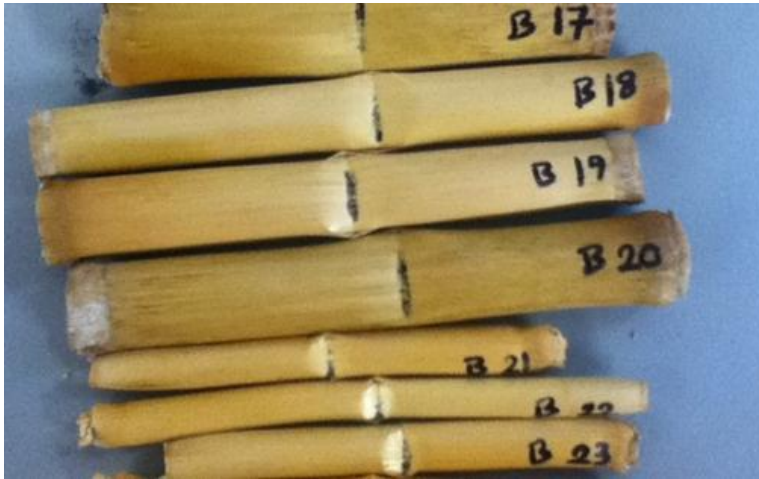
Figure 19. Selected specimens after three-point bending tests
