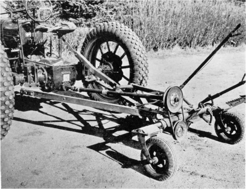
Fig. 10. Showing power drive arrangement and hitch.
