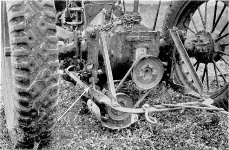
Fig. 3. Belt drive has proven very satisfactory when using a \frac{3}{4} -inch Vee belt. Convenient pulley sizes are 8-inch and 12-inch or 6-inch and 9-inch. Note how frame extension is mounted on drawbar with one \frac{3}{8} -inch bolt. A shield is necessary to keep hay from getting in pulley or on shaft.
