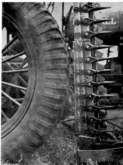
Fig. 8. Extended cutter bar as used during the summer of 1942. The welded extension can be placed on either end of the cutter bar with equal success.
