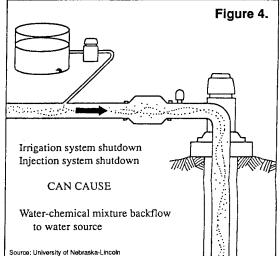
A double, check-valve system is required on the chemical injection line to prevent irrigation water from flowing back through the line and overflowing the chemical supply tank. (Figure 3.)
