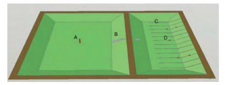
**Figure 1**. Location of the float (A) and weir (B) in the open cell (left), and the sludgelines (C) and temperature loggers (red circles, D) in the covered cell (right).
