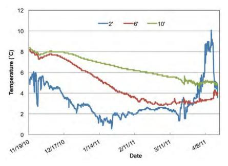
Figure 3. Manure temperatures in the open cell at 0.6 m (2'), 1.8 m (6') and 3 m (10') depths from the surface.
