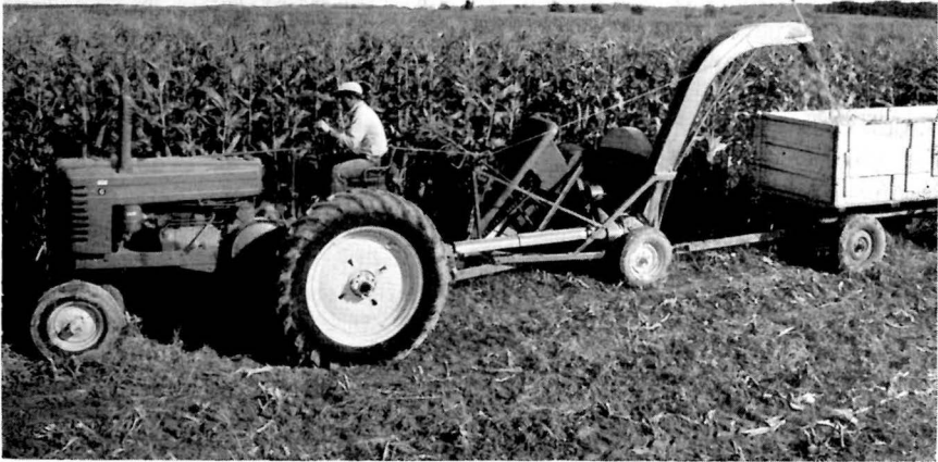
Fig. 1. A field ensilage harvester of the flywheel type, with power-take-off drive
