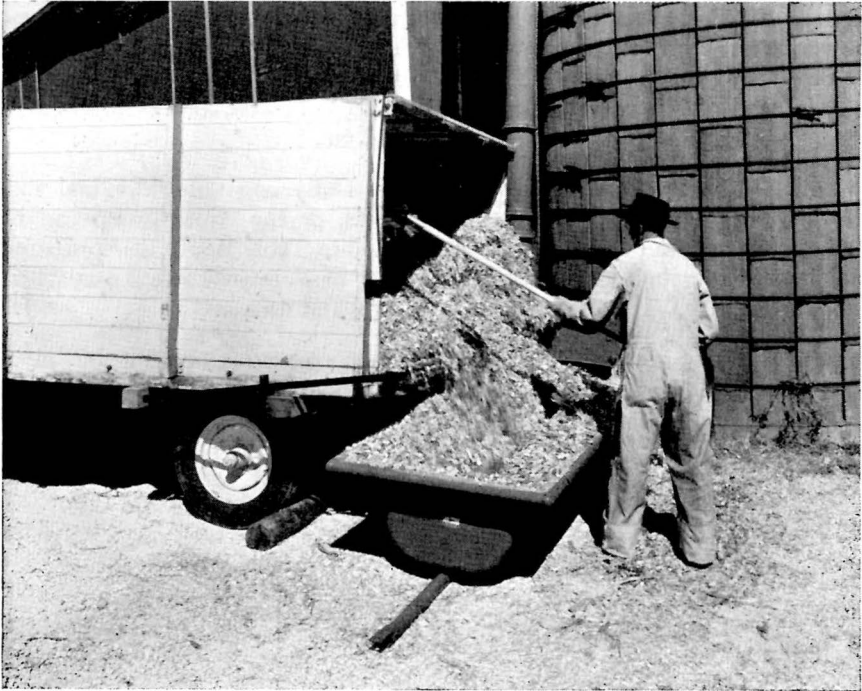
Fig. 5. The blower for ensilage at the silo. Note the low feed hopper and the apron-drive mechanism
