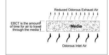
If biofilter space (area) is not limiting, a media depth can be selected and used to find the space needed.
