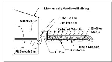
The odorous air is exhausted by a fan from the building and uniformly distributed beneath the biofilter media then rises through the media. Microorganisms attached to the organic media create a biofilm. In this biofilm, they oxidize the biodegradable gases into carbon dioxide, water, mineral salts, and biomass (more microorganisms). The cleaned exhaust air then leaves the biofilter.
