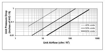
For livestock systems, biofilter media depth is typically 10 to 18 inches. Media depths greater than 18 inches result in excessive pressure drops and greater potential for compaction. Media depths less than 10 inches will dry out more quickly and have a greater potential for air channeling.
