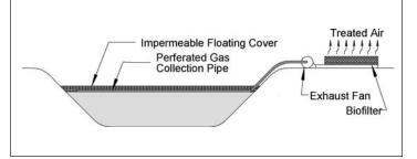
Impermeable covers need to be designed for easy access for operation or maintenance, have a minimum number of joints, and seals at all joints. The corrosive action of sulfides and sulfuric acid must be considered when selecting cover materials and concrete coatings. Overhangs, ledges, or lips on the underside of covers where condensate may collect should be avoided.
