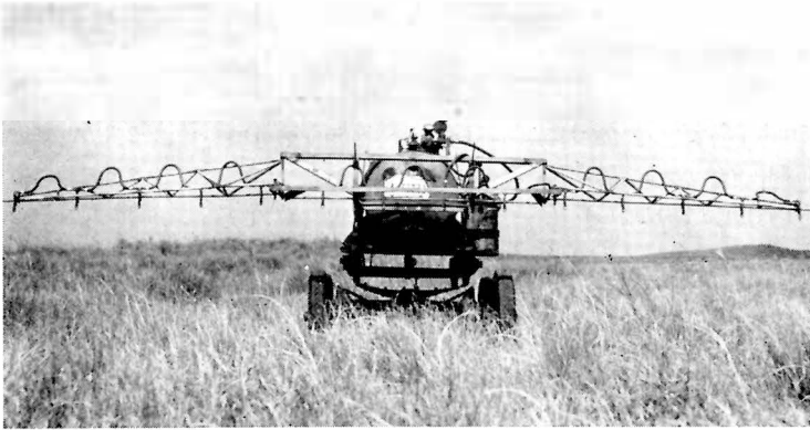
Ground sprayer mounted on 4-wheel trailer for applying foliage sprays to brush on rangeland.
