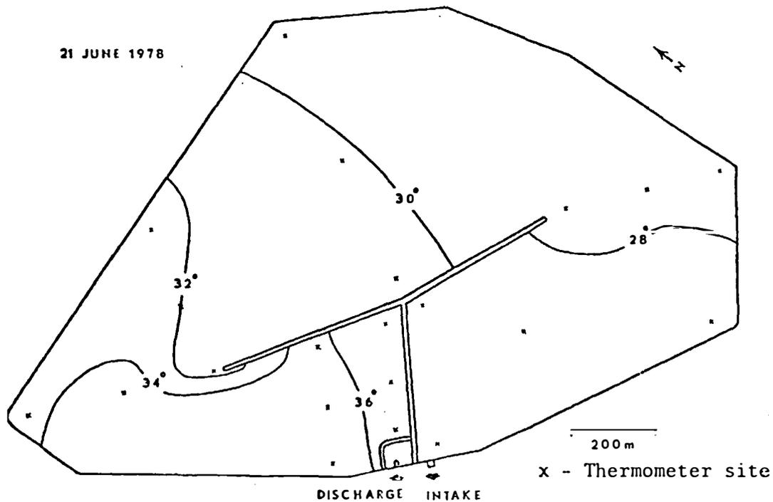
Fig. 7. Temperature (C) at 0.5 m depth, Big Stone Power Plant cooling reservoir, 21 June 1978, during calm conditions.
