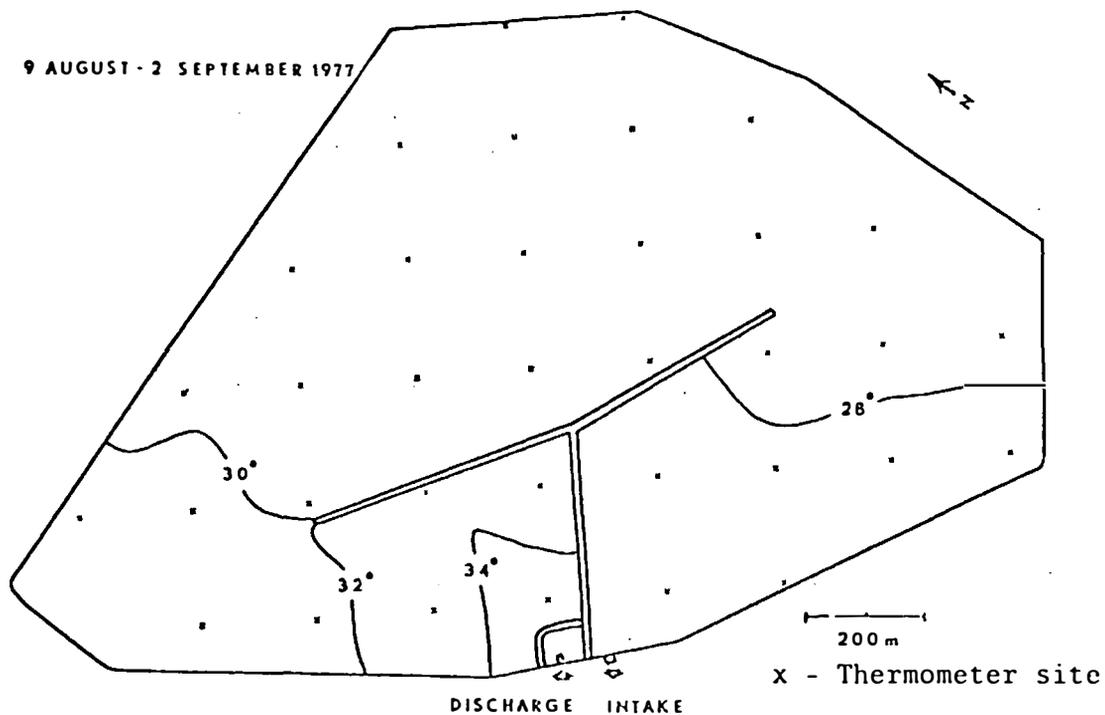
Appendix Fig. 2. Average temperature (C) at 0.5 m depth, Big Stone Power Plant cooling reservoir, South Dakota, 9 August - 2 September 1977. Temperatures shown are mean values of 4 maximum-minimum readings.
