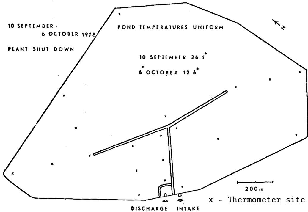
Appendix Fig. 18. Ambient temperature (C) at 0.5 m depth, Big Stone Power Plant cooling reservoir, South Dakota, 10 September and 6 October 1978, with the plant shut down.
