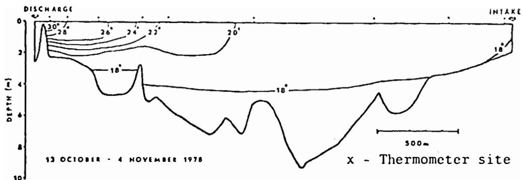
Appendix Fig. 20. Temperature profile (C) of the Big Stone Power Plant cooling reservoir, South Dakota, 13 October - 4 November 1978. Temperatures shown are mean values of 4 ambient readings.
