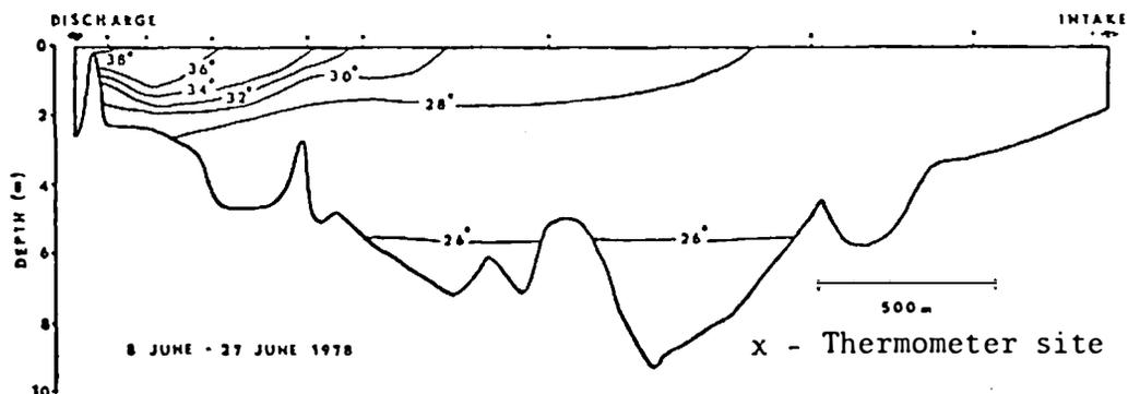
Appendix Fig. 13. Temperature profile (C) of the Big Stone Power Plant cooling reservoir, South Dakota, 8 June - 27 June 1978. Temperatures shown are mean values of 5 ambient readings.
