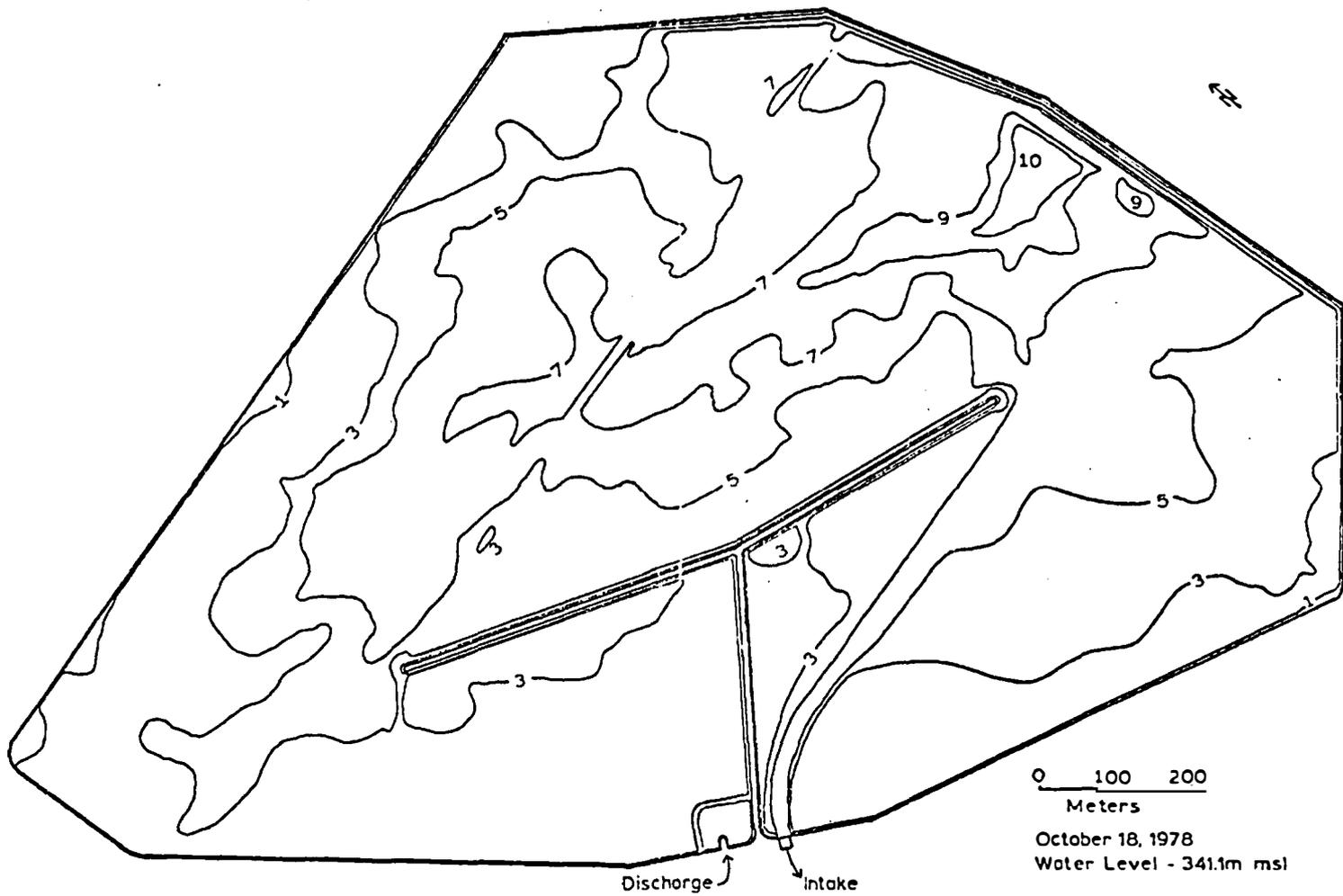
Fig. 1. Big Stone Power Plant cooling reservoir, South Dakota, with depth contours shown at a water level of 341.1 m above mean sea level.
