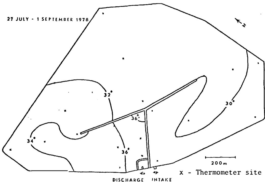
Appendix Fig. 16. Average temperature (C) at 0.5 m depth, Big Stone Power Plant cooling reservoir, South Dakota, 27 July - 1 September 1978. Temperatures shown are mean values of 5 maximum-minimum readings.
