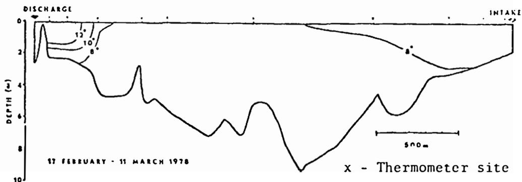
Appendix Fig. 7. Average temperature profile (C) of the Big Stone Power Plant cooling reservoir, 17 February - 11 March 1978. Temperatures shown are mean values of 4 ambient readings.
