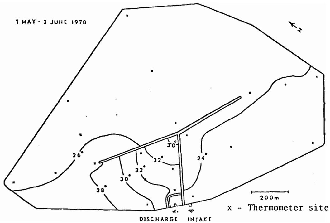
Appendix Fig. 10. Average temperature (C) at 0.5 m depth, Big Stone Power Plant cooling reservoir, 1 May - 2 June 1978. Temperatures shown are mean values of 4 maximum-minimum readings.
