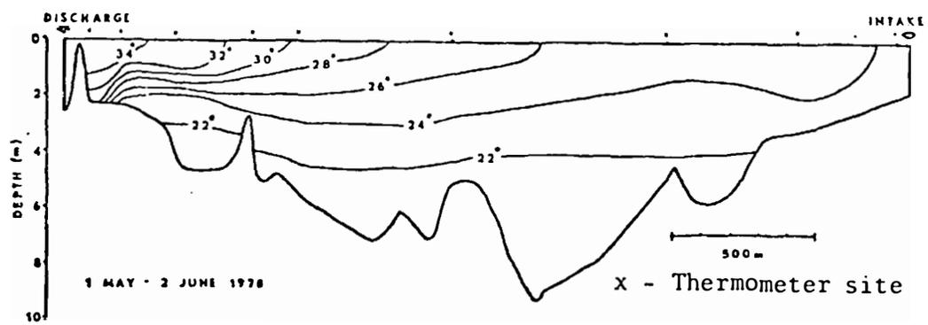
Appendix Fig. 11. Temperature profile (C) of the Big Stone Power Plant cooling reservoir, South Dakota, 1 May - 2 June 1978. Temperatures shown are mean values of 4 ambient readings.
