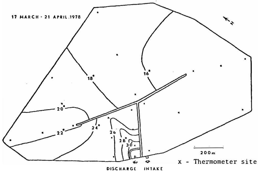
Appendix Fig. 8. Average temperature (C) at 0.5 m depth, Big Stone Power Plant cooling reservoir, South Dakota, 17 March - 21 April 1978. Temperatures shown are mean values of 6 ambient readings.
