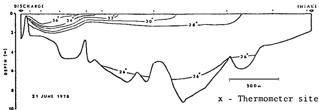
Fig. 8. Temperature profile (C) of the Big Stone Power Plant cooling reservoir, 21 June 1978, during calm conditions.
