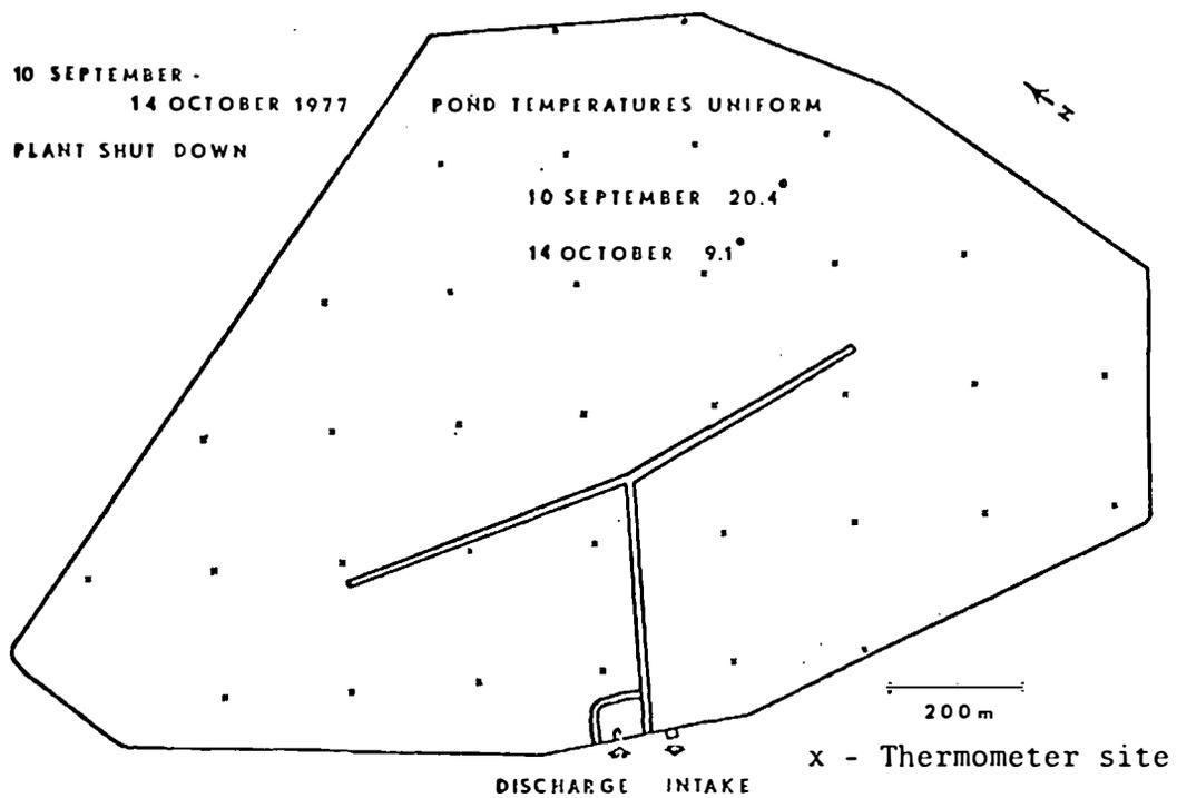
Appendix Fig. 3. Ambient temperature (C) at 0.5 m depth, Big Stone Power Plant cooling reservoir, South Dakota, 10 September and 14 October 1977, with the power plant shut down.
