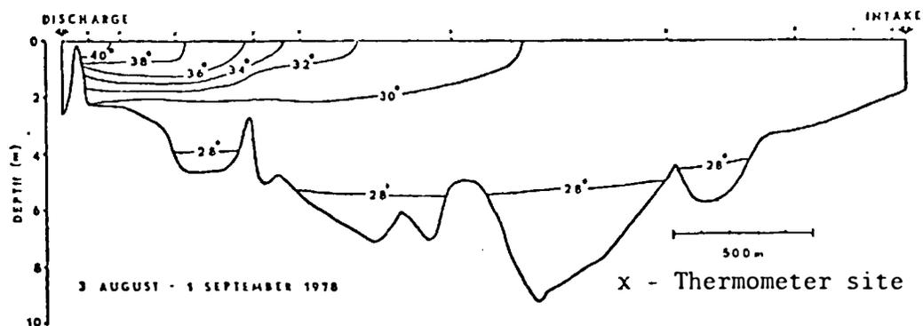
Appendix Fig. 17. Temperature profile (C) of the Big Stone Power Plant cooling reservoir, South Dakota, 3 August - 1 September 1978. Temperatures shown are mean values of 5 ambient readings.
