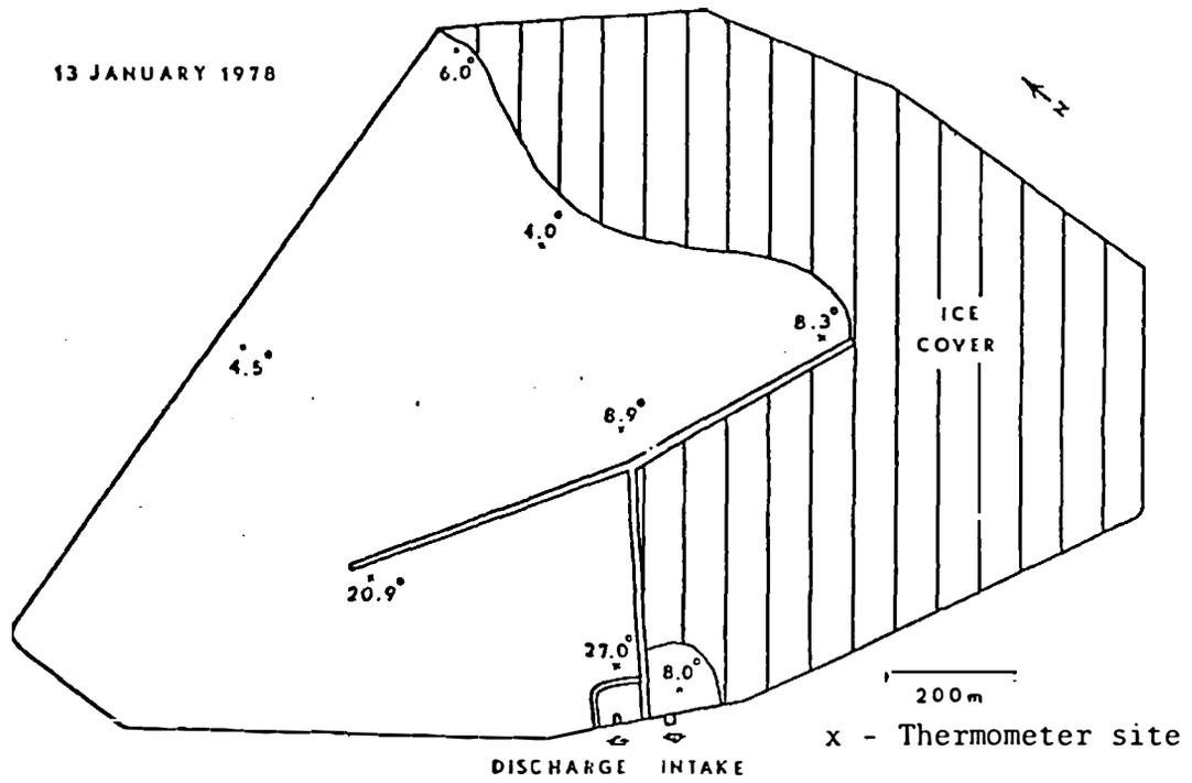
Appendix Fig. 5. Ambient temperature (C) at 0.5 m depth, Big Stone Power Plant cooling reservoir, South Dakota, 13 January 1978.
