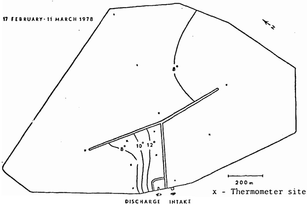
Appendix Fig. 6. Average temperature (C) at 0.5 m depth, Big Stone Power Plant cooling reservoir, South Dakota, 17 February - 11 March 1978. Temperatures shown are mean values of 4 ambient readings.
