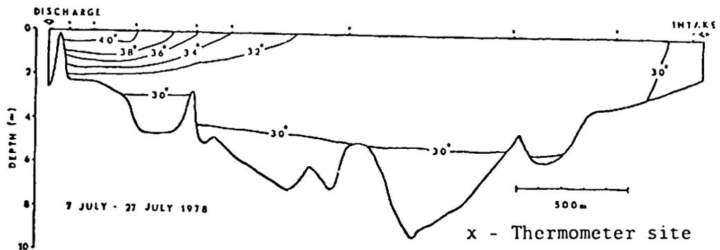
Appendix Fig. 15. Temperature profile (C) of the Big Stone Power Plant cooling reservoir, South Dakota, 7 July - 27 July 1978. Temperatures shown are mean values of 4 ambient readings.
