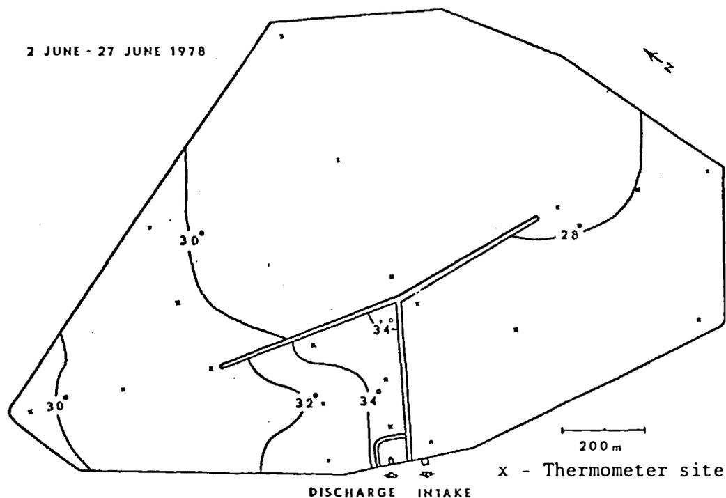
Appendix Fig. 12. Average temperature (C) at 0.5 m depth, Big Stone Power Plant cooling reservoir, South Dakota, 2 June - 27 June 1978. Temperatures shown are mean values of 4 maximum-minimum readings.
