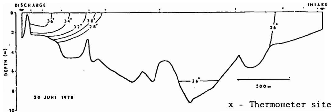
Fig. 6. Temperature profile (C) of the Big Stone Power Plant cooling reservoir, South Dakota, 20 June 1978, during 32 km/hr northwest winds.
