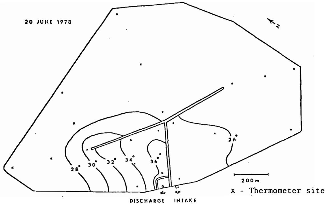
Fig. 5. Temperature (C) at 0.5 m depth, Big Stone Power Plant cooling reservoir, South Dakota, 20 June 1978, during 32 km/hr northwest winds.
