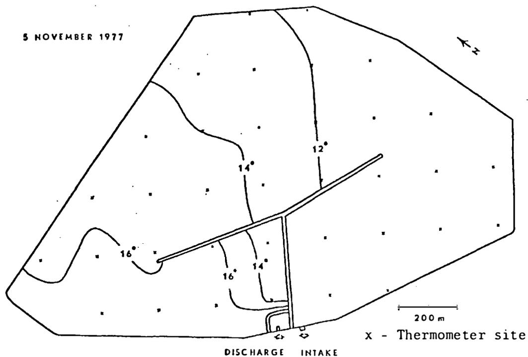
Appendix Fig. 4. Ambient temperature (C) at 0.5 m depth, Big Stone Power Plant cooling reservoir, South Dakota, 5 November 1977.
