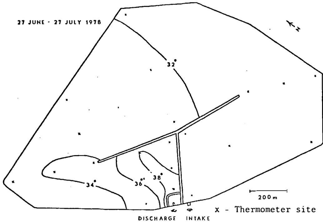
Appendix Fig. 14. Average temperature (C) at 0.5 m depth, Big Stone Power Plant cooling reservoir, South Dakota, 27 June - 27 July 1978. Temperatures shown are mean values of 4 maximum-minimum readings.
