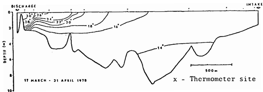
Appendix Fig. 9. Temperature profile (C) of the Big Stone Power Plant cooling reservoir, South Dakota, 17 March - 21 April 1978. Temperatures shown are mean values of 6 ambient readings.
