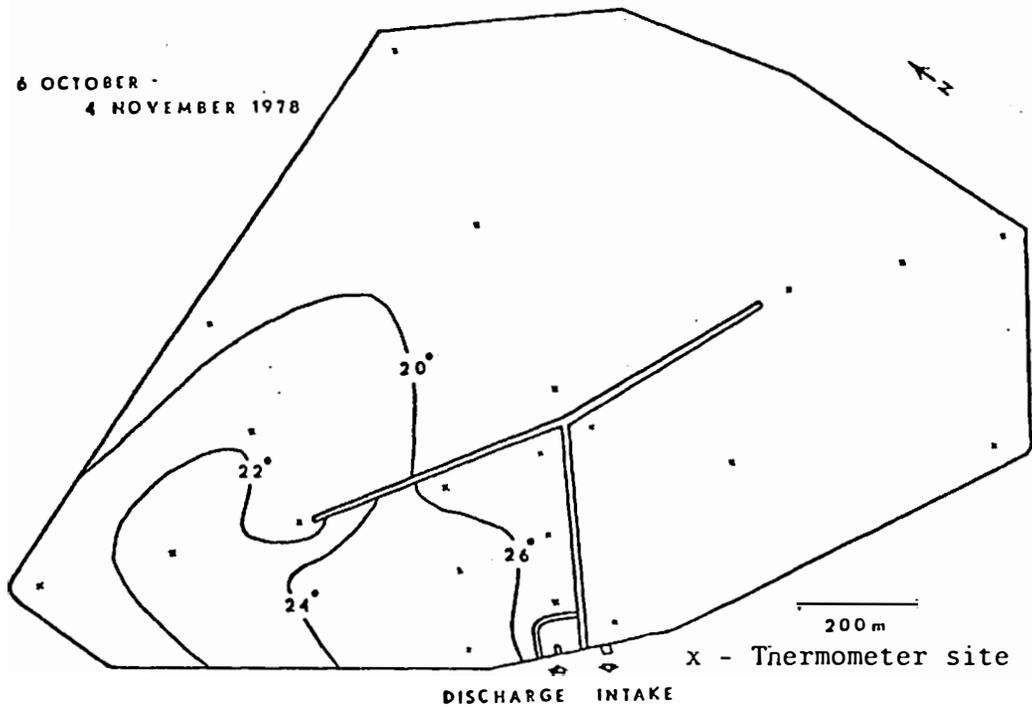
Appendix Fig. 19. Average temperature (C) at 0.5 m depth, Big Stone Power Plant cooling reservoir, South Dakota, 6 October - 4 November 1978. Temperatures shown are mean values of 4 maximum-minimum readings.
