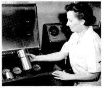
This machine aids in testing the ability of various detergents to remove soil from fabrics.
