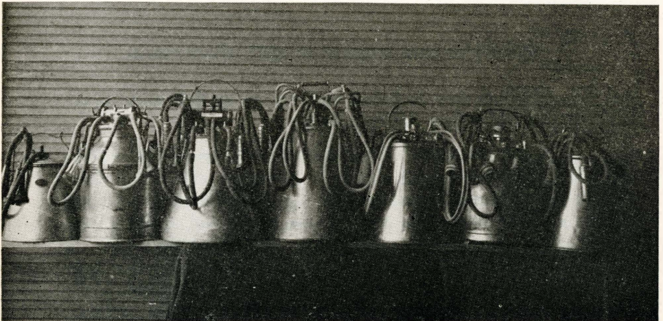
View of all of the milking machines in the experiment. From left to right they are: Hinman, Waterloo Boy, Perfection, Empire, Calfway, B. L. K., and Sharples.
