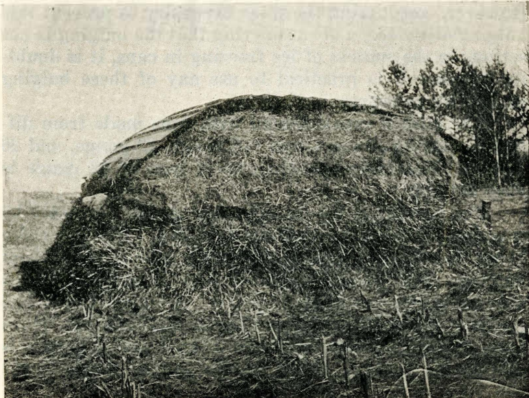
FIGURE VII. Pile of ice stored on top of ground from which only 10 per cent of ice stored was recovered for actual use.
