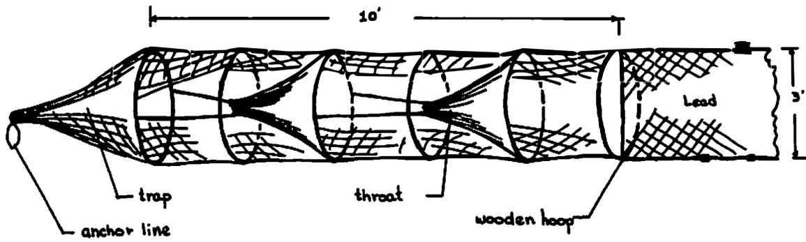
Figure 1. -- Schematic drawing of one-half of a pocket-net.
