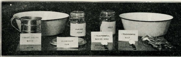
Fig. 6.—Cleaning silver by electrolysis.
