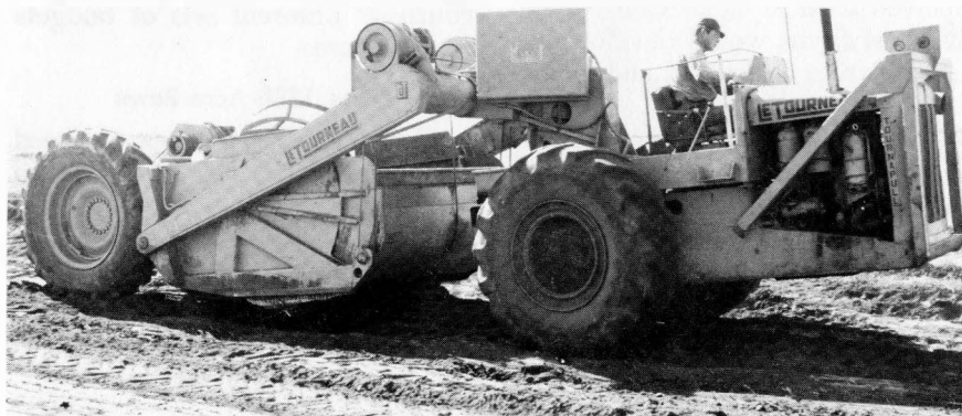
Land smoothing, required for gravity irrigation, is one costly but necessary operation done initially by heavy equipment. Deep cuts will require recommended practices for fertility restoration. Where leveling is not economical, sprinkler irrigation may be used. (Bureau of Reclamation Photo.)
