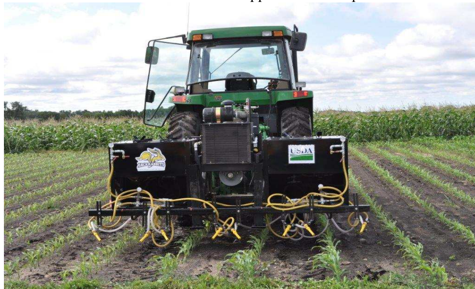
Figure 2-1. In-row grit application applied in Morris, MN in 2013 and 2014 was made with a four-row applicator developed at SDSU.
