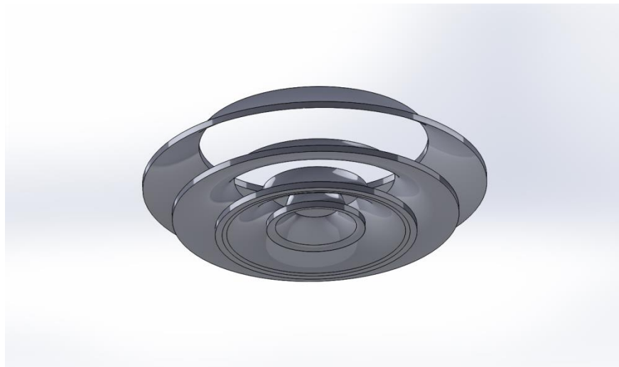
Figure 5: Solidworks Model of Round Diffuser; 45 degree throw angle, 4 shells
