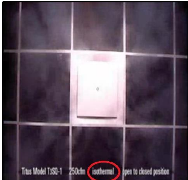
Figure 148: Smoke test showing air flow patterns from diffuser [14]
