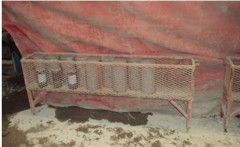
Fig. 3. Creep samples placed next to girder bed prior steam curing.
