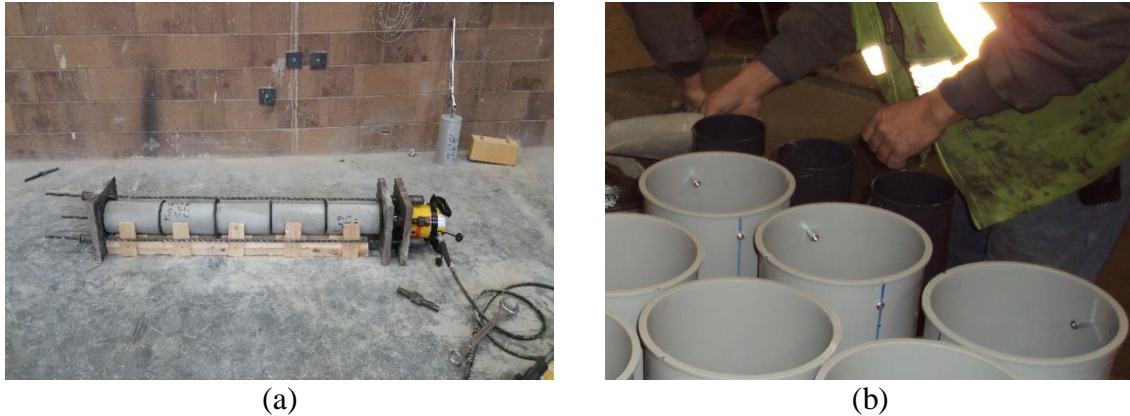
Fig. 5. Creep test set up: (a) Loaded creep frame; (b) Modified cylinder with brass inserts on both sides.
