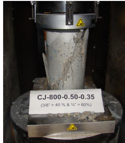
b) Diagonal crack of cylinder
