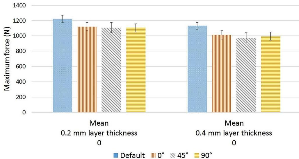
Fig. 16. Comparison of the A-frame tensile test results.
