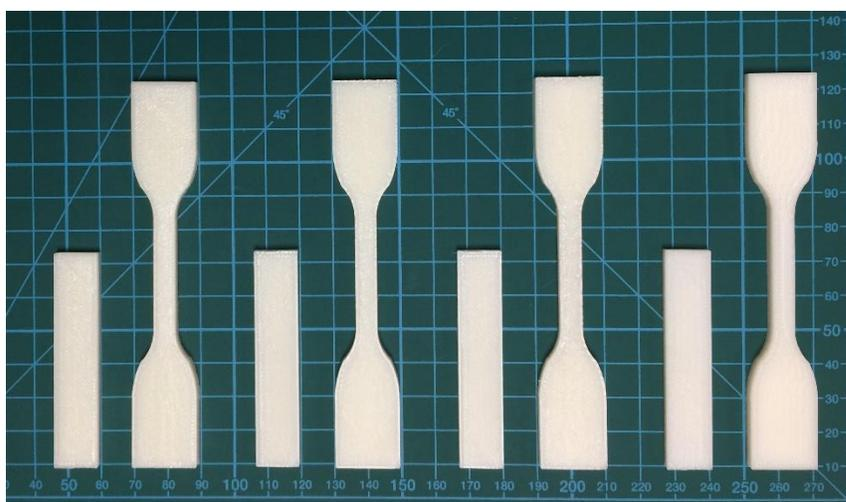
Fig. 9. Tensile and flexural test specimens made of irradiated ABS filament. From right to left: control sample, samples exposed to 1 kGy, 5 kGy and 10 kGy.
