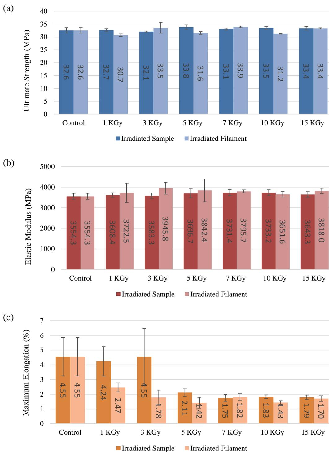
Fig. 17. Graphical comparison of tensile test results for CF-ABS samples. (a) ultimate strength, (b) elastic modulus and (c) maximum elongation.
