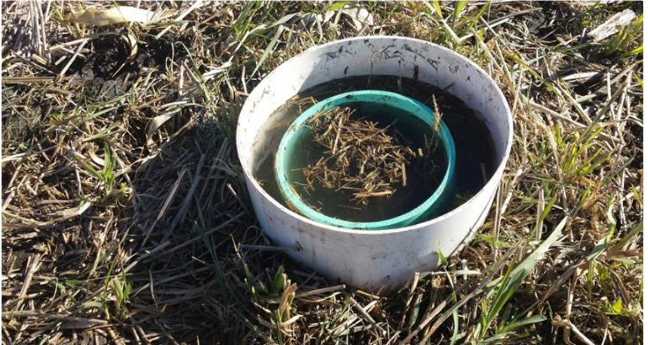
Figure A.2 Double ring infiltration rate method for measuring water infiltration
