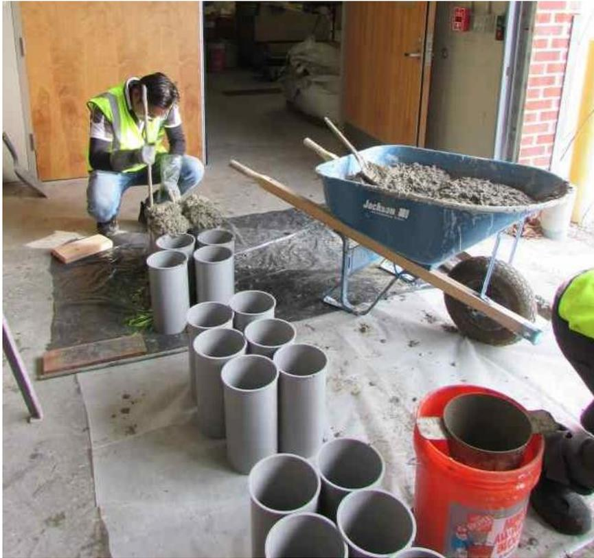
**Figure 2-5. Casting of concrete cylinders**
