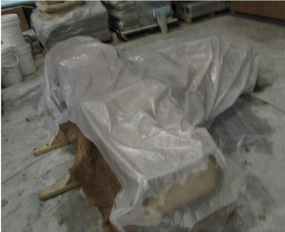
**Figure 4-19. Curing of beam-column test specimen**
