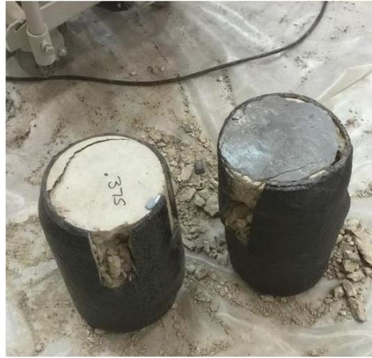
(b) Extracting Rubber to determine thickness
