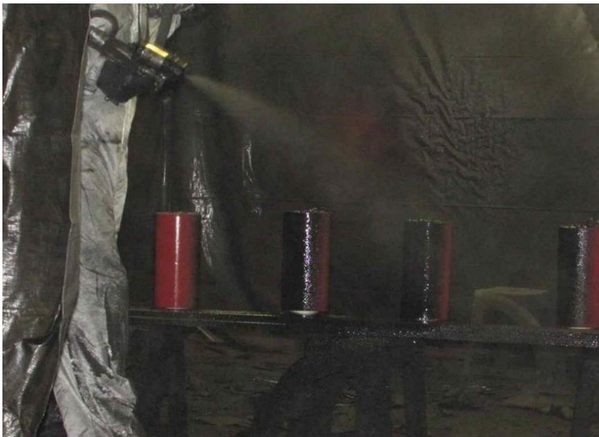
**Figure 2-8. Spraying rubber on concrete specimens**
