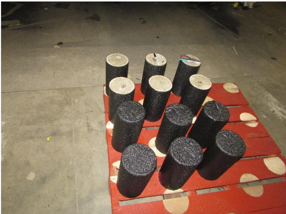
**Figure 2-10. Rubber-coated concrete specimens**
