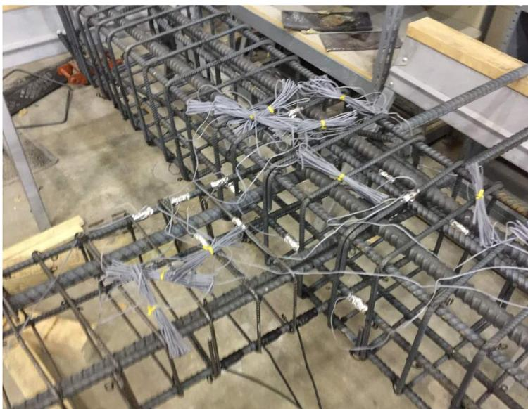
**Figure 4-25. Installation of strain gauges in beam-column specimen**
