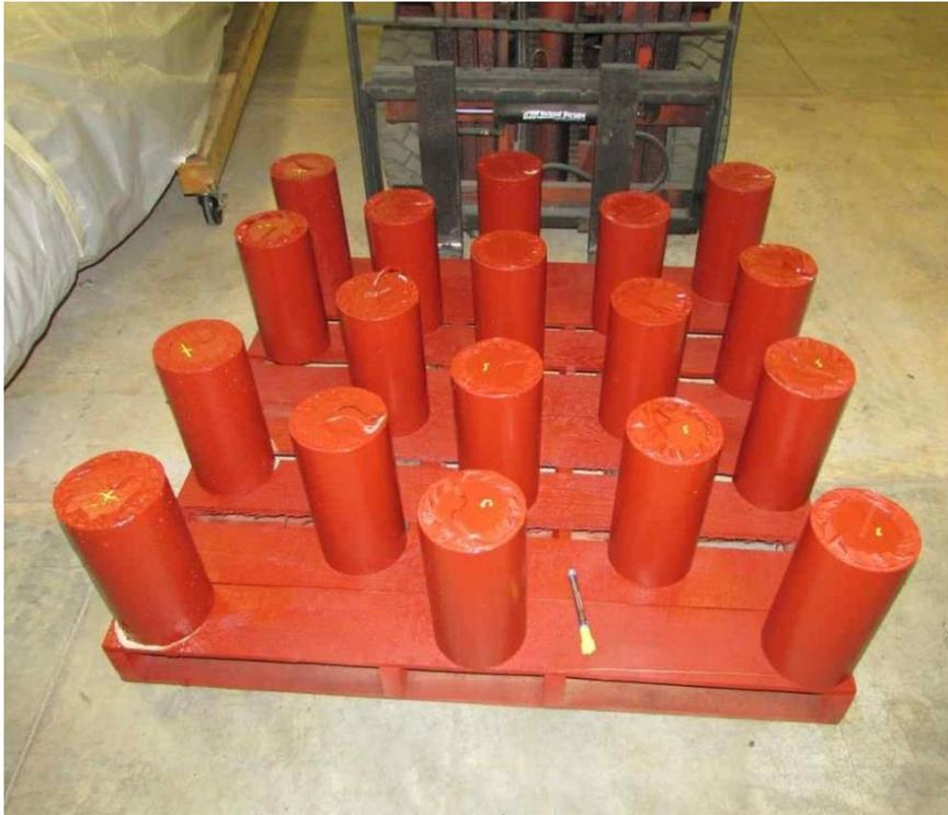
**Figure 2-7. Thin layer of base coat on concrete**
