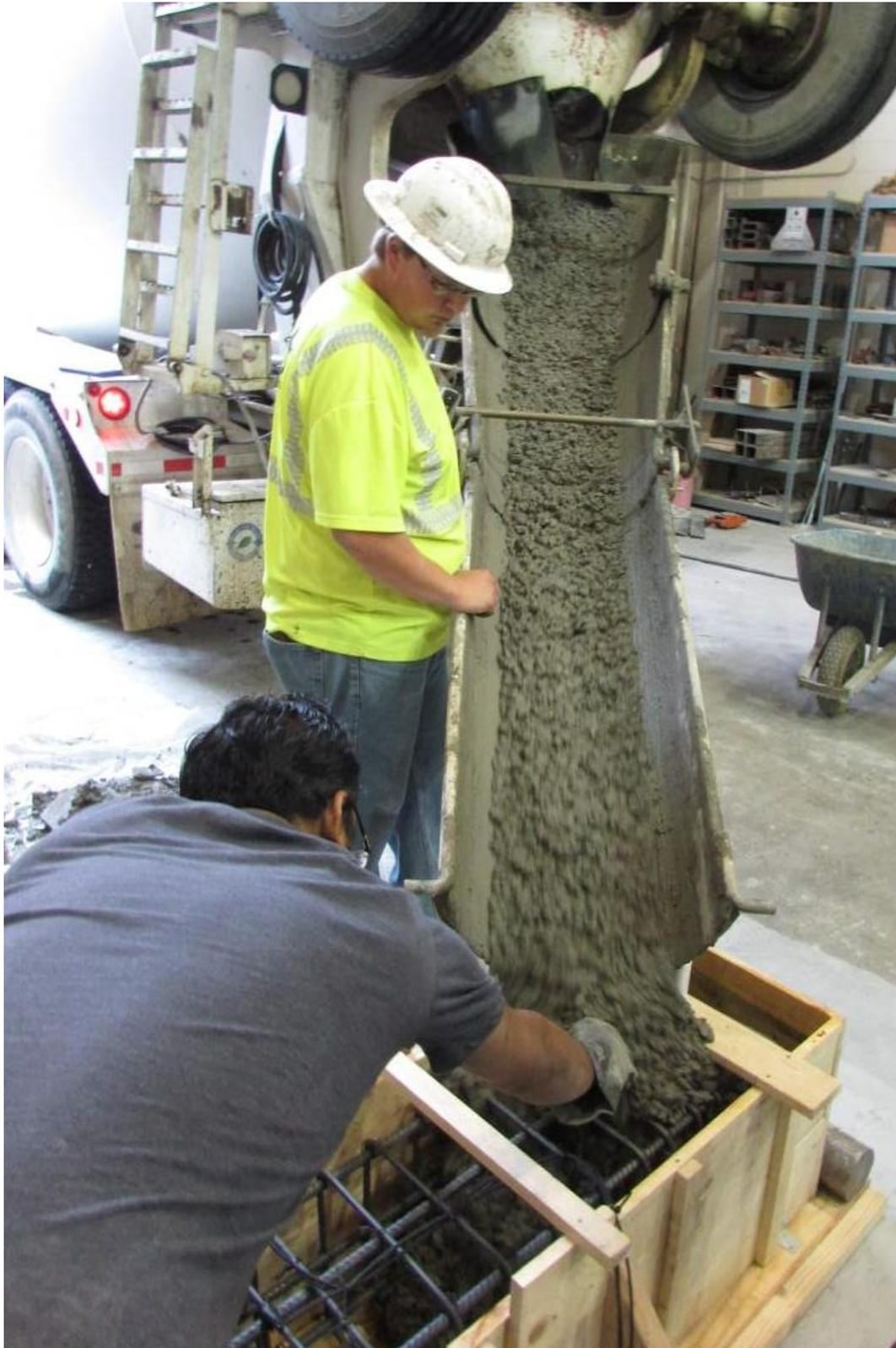
Figure 4-18. Concrete pouring for beam-column test specimen
