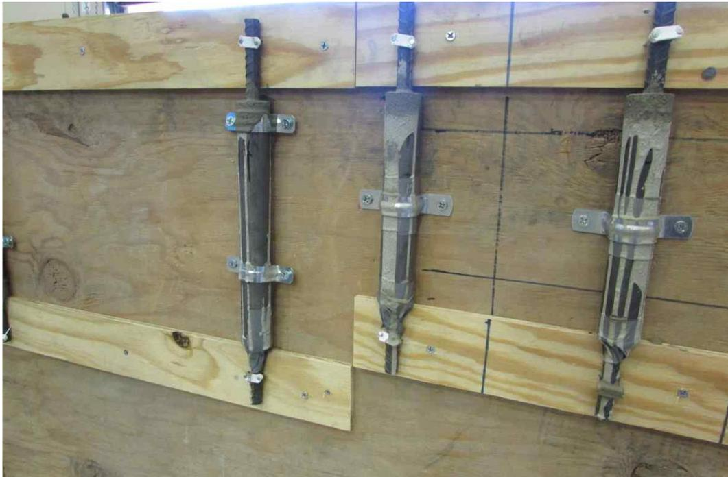
**Figure 3-14. BRR specimens after pouring non-shrink grout**
