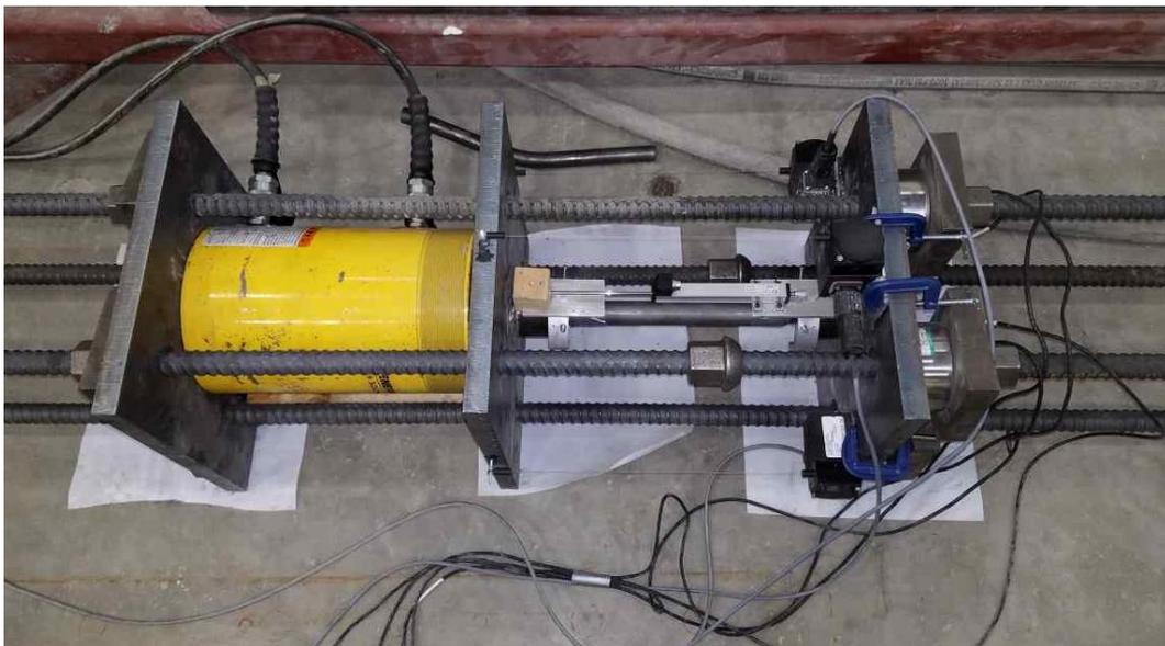
**Figure3-16. Photograph of BRR test setup**
