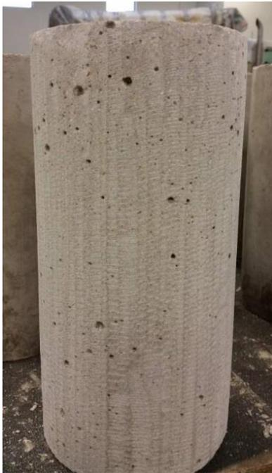
**Figure 2-6. Concrete surface preparation for two specimens**
