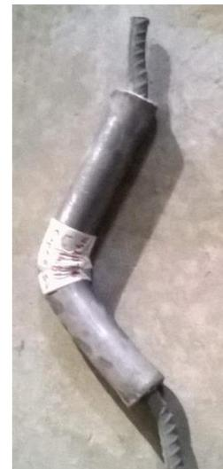
(b) BRR device at failure
