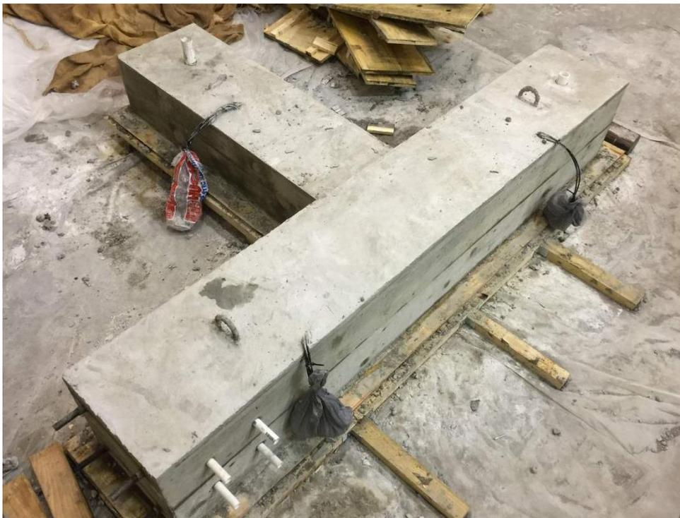
**Figure 4-20. Beam-column test specimen**
