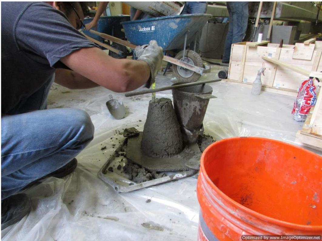
Figure 4-17. Slump of ready mix concrete
