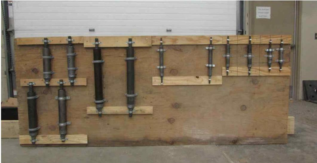
**Figure 3-13. Construction of BRR specimens**
