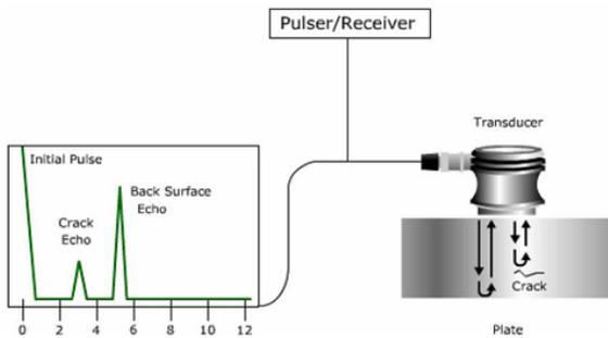
**Figure 1: Wave Reflection and Receiver Signal [4]**
