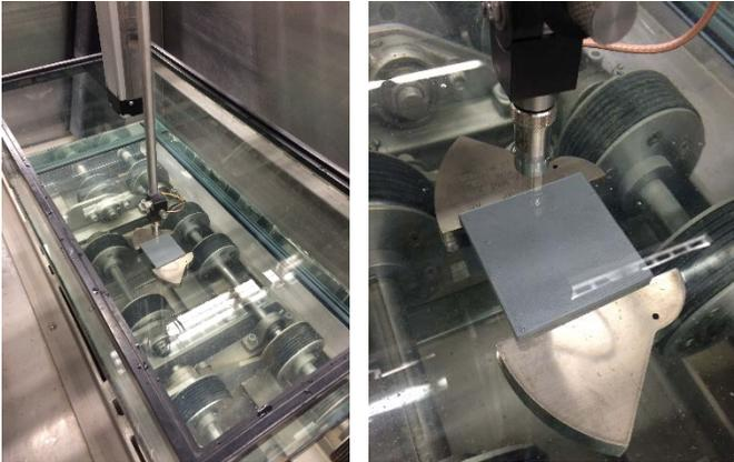
**Figure 5: Ultrasound Tank Setup for C-scan (left), Close up of Specimen Setup (right)**
