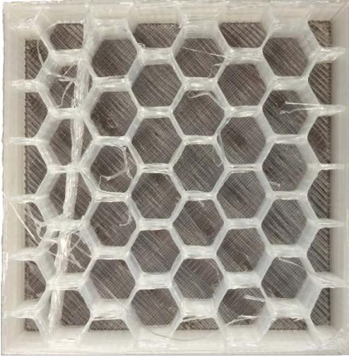
**Figure 11: 30% Infill Specimen Cross Section**
