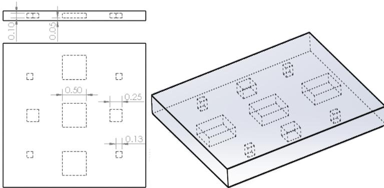
**Figure 4: Internal Features Specimen**
