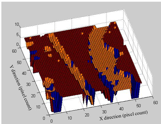
**Figure 7: Initial thickness test (in  $\mu\text{s}$ ) for backside surface geometry detection**
