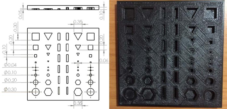
**Figure 3: Precision Evaluation Specimen**
