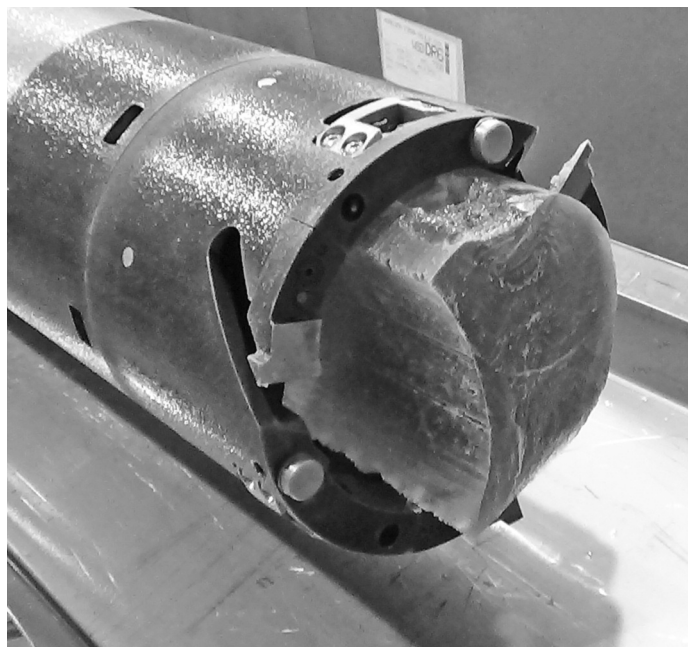
This chunk of ice has made history. A National Science Foundation-funded replicate core drilling team was able to retrieve cylinders of ice from the original ice core hole while leaving the borehole intact.
