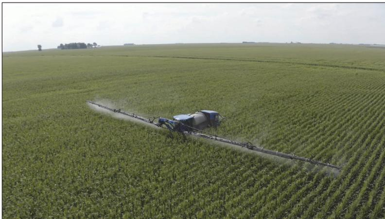
**Figure 2.** Photo of a high-clearance front boom sprayer operating in a canopied corn field. Under these conditions, VSN Full Canopy uses radar sensors instead of a stereo camera to detect crop rows.
