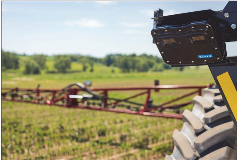
**Figure 1.** Photo of a VSN (black box) positioned in front of the right front wheel on a rear boom sprayer. The stereo camera lenses are behind the clear windows of the VSN enclosure.
