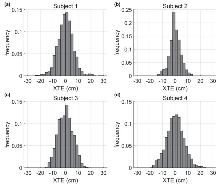
**Figure 7. Histograms of XTE measurement frequency in 2 cm bins. Both steering types are included for each subject. There were 6226, 709, 9426, and 6938 data points for subjects 1 to 4, respectively.**
