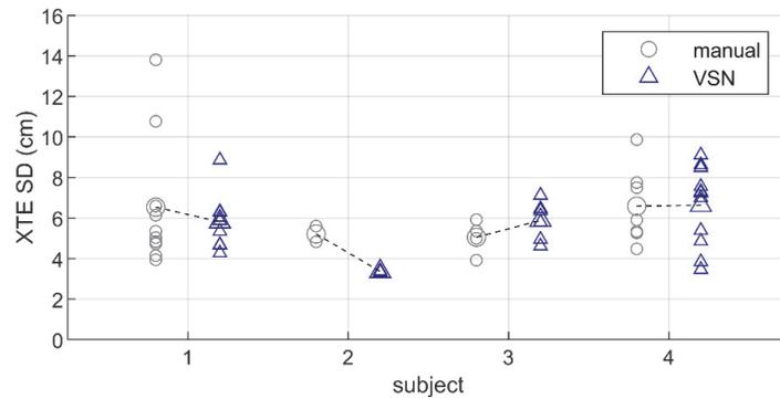
**Figure 6. Individual value plot of cross-track error standard deviation (XTE SD) for each steering type and subject. Each smaller shape represents the measurement of one pass, and the larger shape represents the steering type mean for each subject.**
