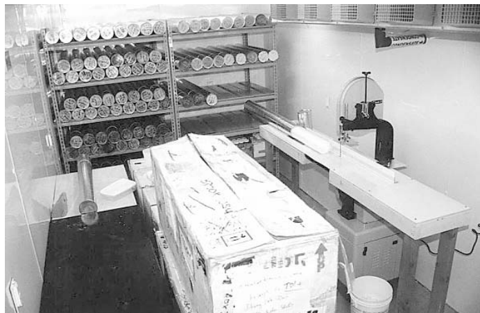
An interior view of the cold lab showing stored ice core samples and saw for preparing samples.
