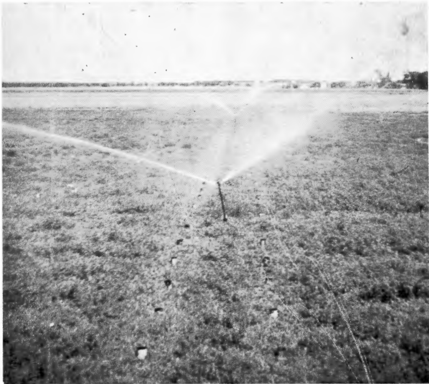
Arrangement used to determine the effect of wind on water distribution.
