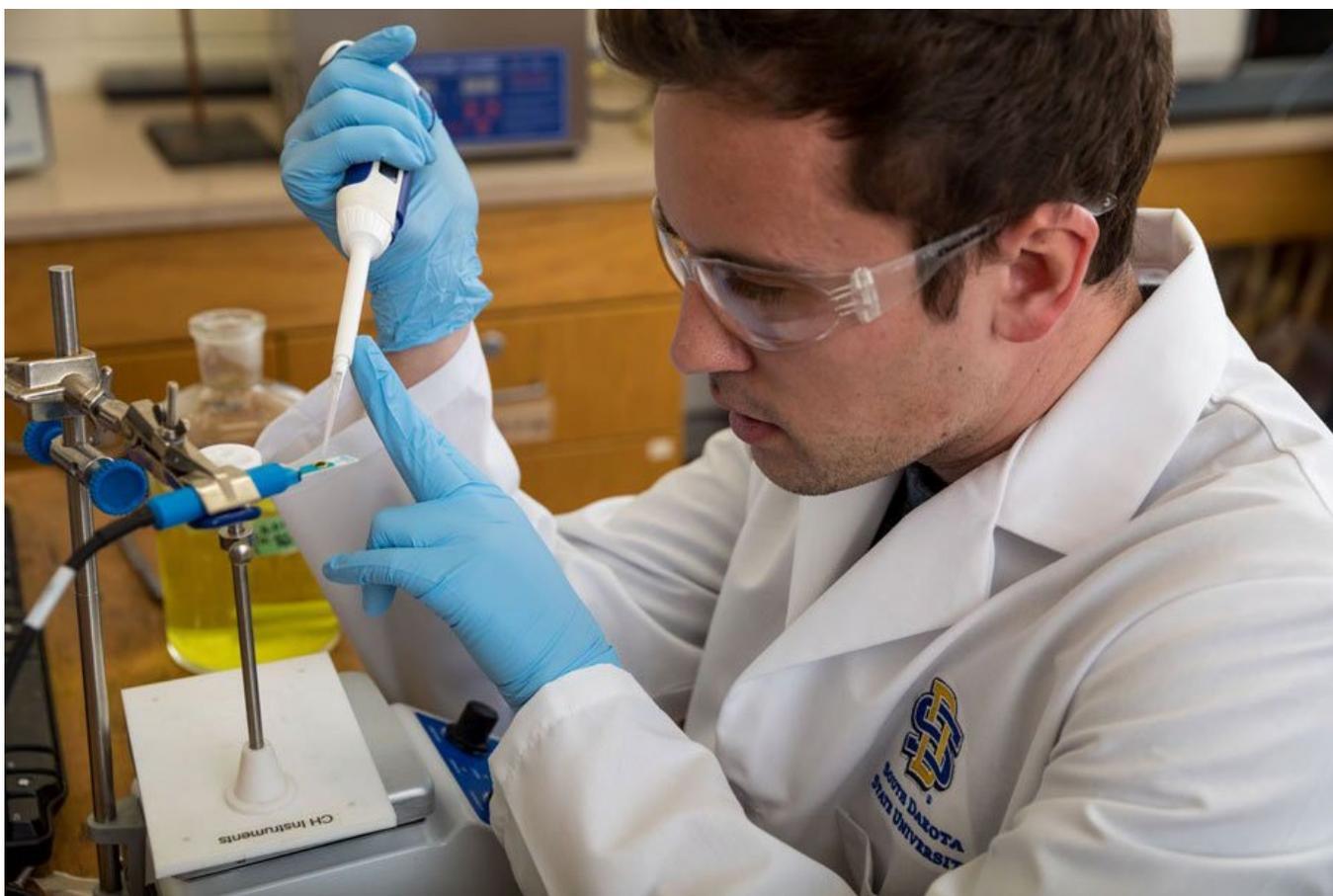
*Graduate student Matthew Hummel uses a known sample to calibrate the biosensor, which is designed to detect viral DNA in animal and environmental samples. When the viral DNA attaches to the bioprobe, increases the resistance of the graphene.*
