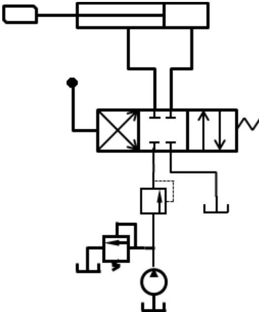
**Figure 3: Pressure Control Circuit Diagram**
