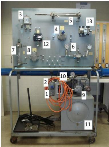
**Figure 1: Hydraulic Test Bench Components**
