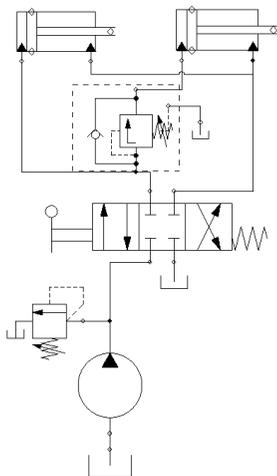
**Figure 6: Sequencing Control Circuit**
