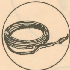
A "SNAKE" MADE OF STEEL FOR USE IN PUSHING THROUGH SLUDGE IN THE DRAIN
