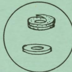
Packing or new washers for use in stopping leaks in the flush tank
