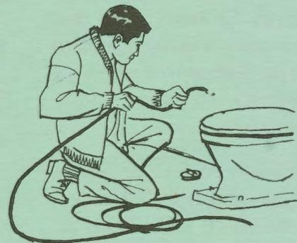
The best way to clean a clogged drain is with the metal “snake.” The snake can be pushed down the drain through the toilet bowl or through the clean-out plug near the toilet, or through the vent pipe on the roof.
