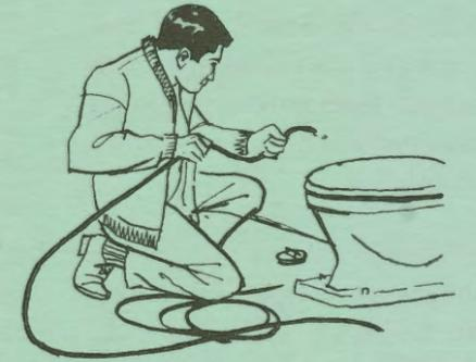
Sometimes objects like toys, pencils or sanitary napkins get in the toilet by mistake. In this case the plunger may not be of much help. Make a hook on the end of a wire. Poke the wire with the hook into the stool and try to pull out the object.
