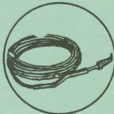
A "snake" made of steel to use in pushing sludge through the drain
