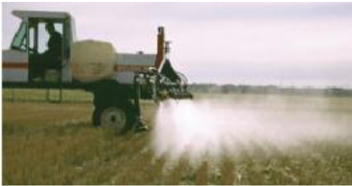
Figure 2. Conventional flat fan spray tips at 40 psi. (Wolf)
