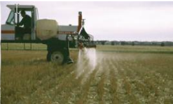
Figure 3. Air induction nozzles at 70 psi. (Wolf)
