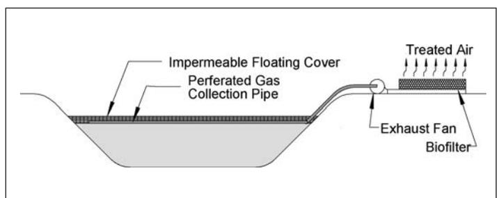
Impermeable covers need to be designed for easy access for operation or maintenance, have a minimum number of joints, and seals at all joints. The corrosive action of sulfides and sulfuric acid must be considered when selecting cover materials and concrete coatings. Overhangs, ledges, or lips on the underside of covers where condensate may collect should be avoided.
