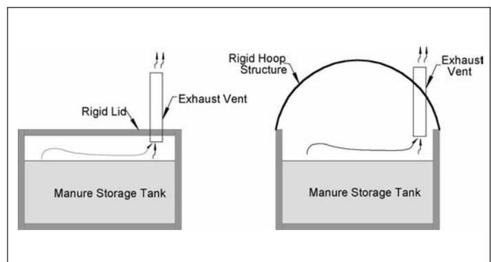
**Figure 2. System to remove and treat biogas from manure storage using an impermeable cover and biofilter.**
