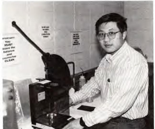
Dr. C. Y. Wang uses an electronic balance to accurately weigh a sample of soy flour. The material is the basis for soy isolate, which is 90 percent protein.
