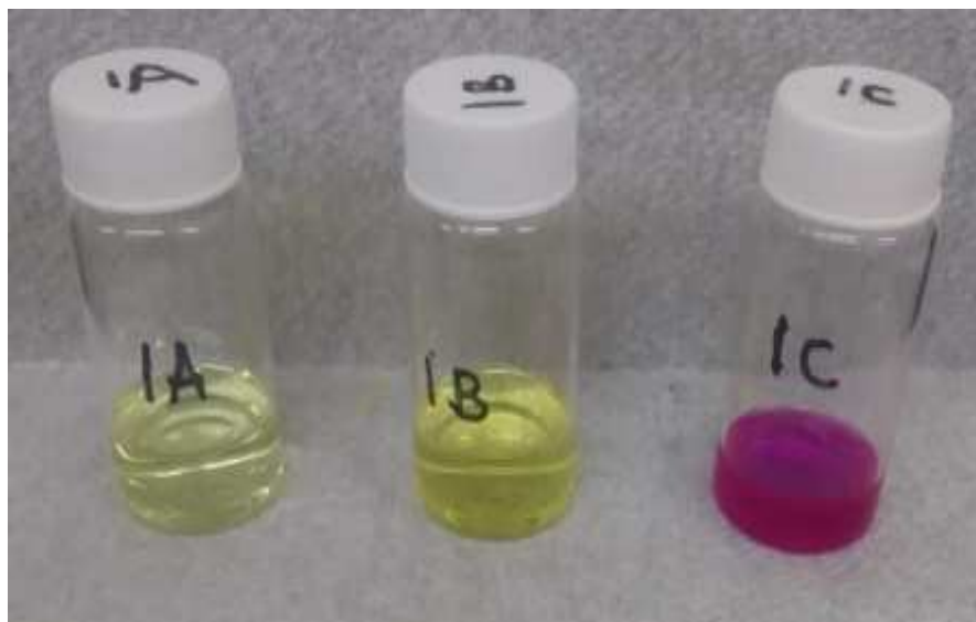
Figure 4.3. Light yellow, yellow and purple color of 4-nitroaniline, N,N-diethyl-4-nitroaniline and Nile red dyes dissolved in DESs.
