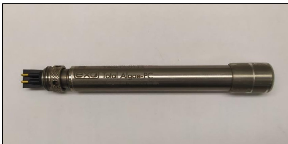
Figure 29. The Total Algae-PC sensor used in EXO2 sonde during data collection. Photo by Sumit Kumar Ghosh.
