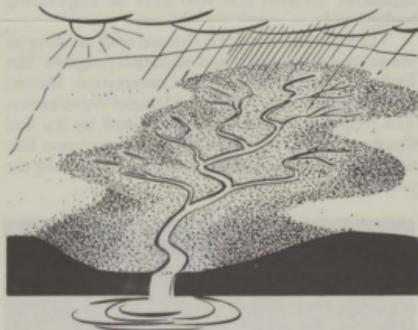
The drainage pattern of a watershed is illustrated in this diagram. In effective watershed development, the total area must be considered, uplands, stream channels, and lowlands.
