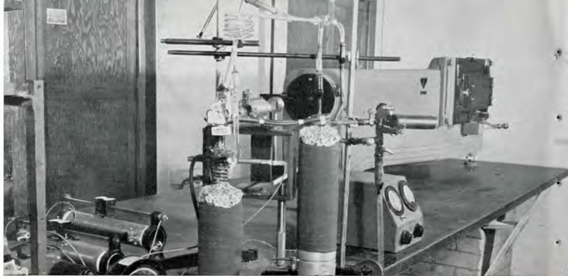
Equipment for measuring hyperfine structure in atomic spectra.
