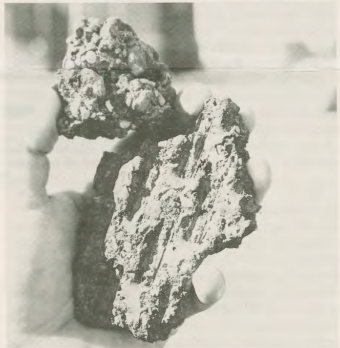
Figure 2. These incrustations were caused by precipitation of material carried up to the screen in solution.
