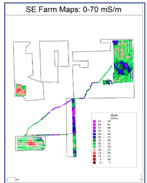
The TSM sensor was driven across several fields in April- early May. The TSM sensor seemed to be picking up general field patterns that could be related to apparent electrical conductivity readings. It even appeared to pickup a disposal area in the NE Quarter connected to the old Farmstead. Large conductance readings of four hundred mS/m appeared right over the small area.
