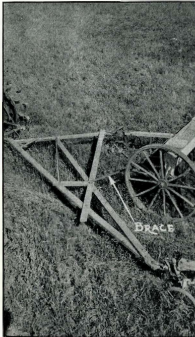
Fig. 2. —The Two-Implement Hitch For Drills, Field Cultivators or Disks
