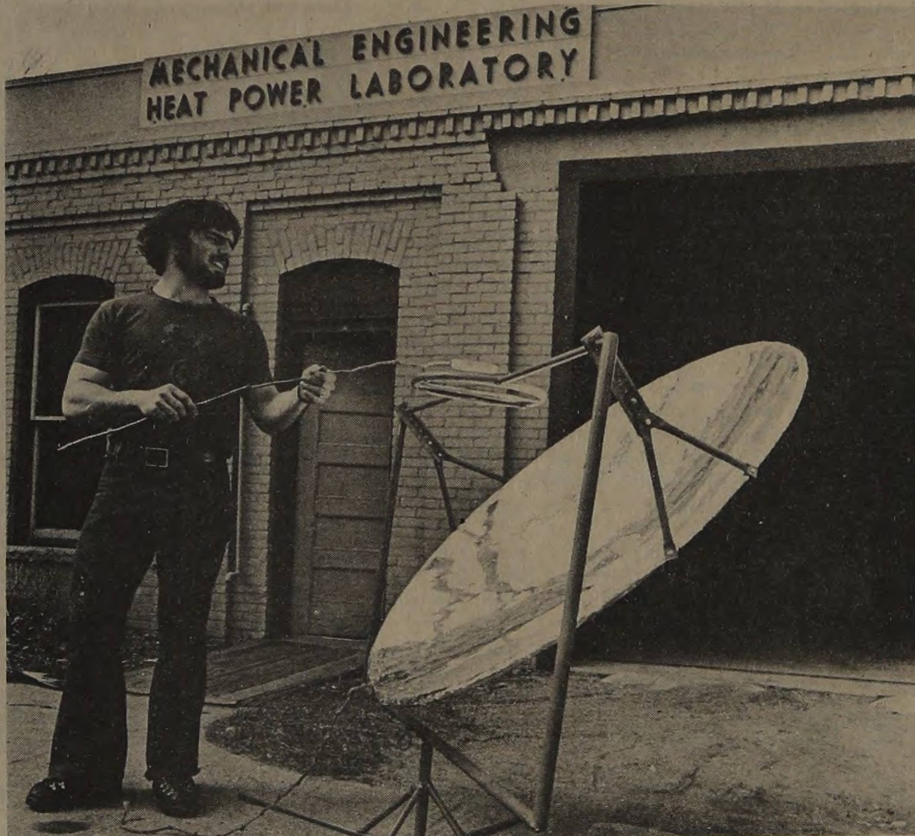
Roger Huber, mechanical engineering senior, cooks a hotdog Monday with his parabolic reflector for a
