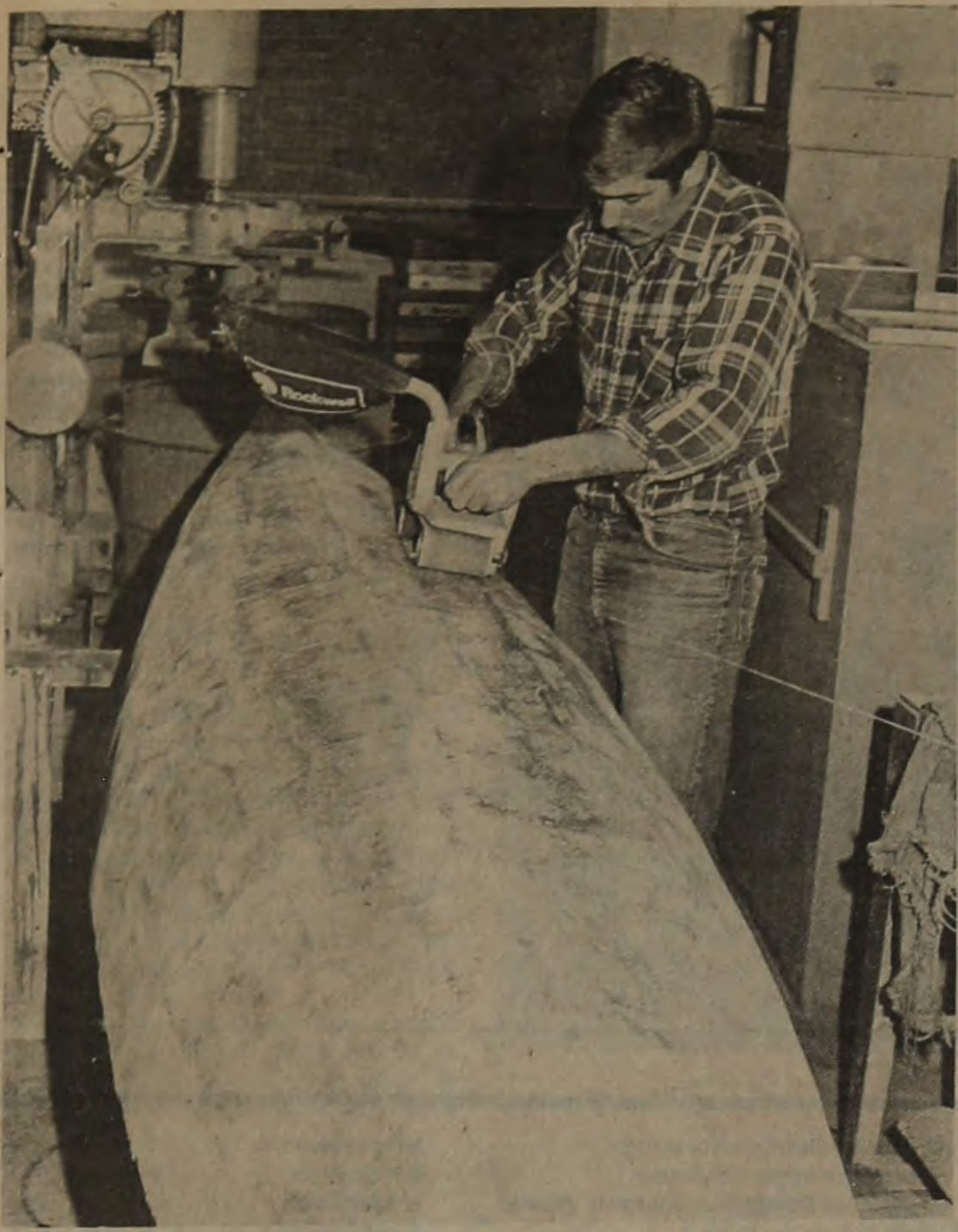
Jim Krier adds some of the final touches to the concrete canoe.
