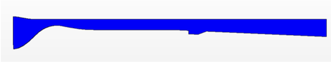
Figure 8: StarCCM+ CAD Model of Supersonic Combustion Chamber
