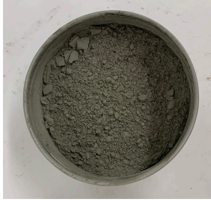
Figure 3.2. Portland cement type I used in this study.
