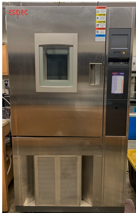
Figure 3.9 A photographic view of the environmental chamber used for the freeze-thaw test.
