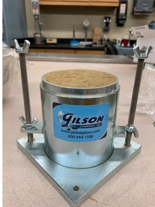
Figure 3.8 Photographic view of the Proctor mold and the compacted soil sample.
