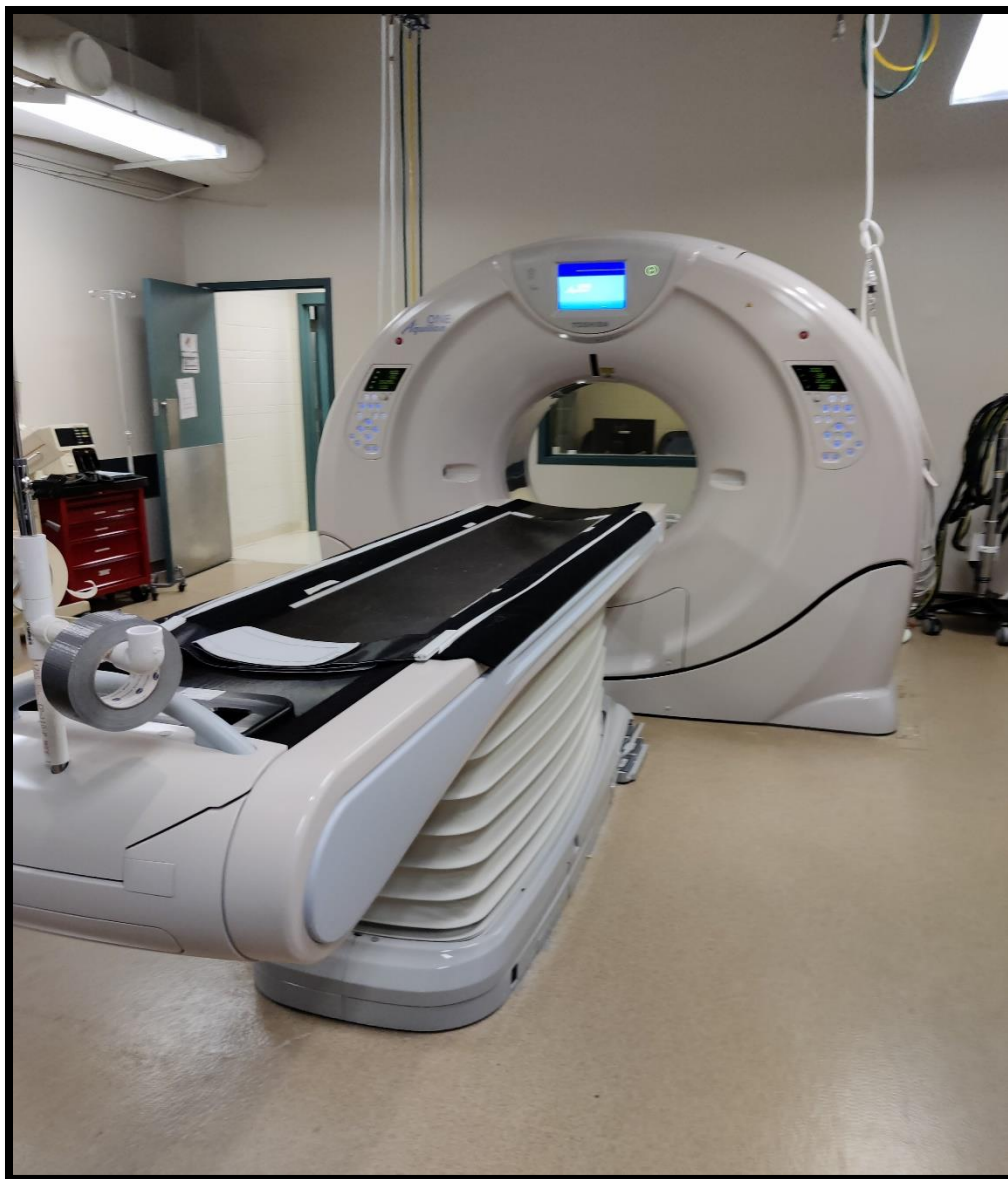
Appendix 3.C. X-ray Computed Tomography scanner used for the scanning of soil cores at University of Missouri, Columbia, USA.
