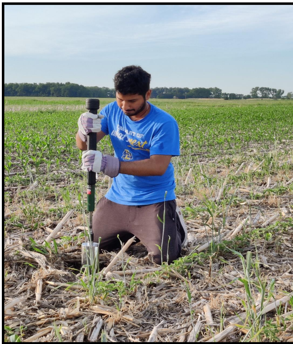
Appendix 3.A. Collecting plexiglass core samples using soil core sampler.
