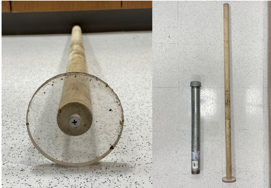
Figure 3: Photos of tamping system used to pack woodchip samples
