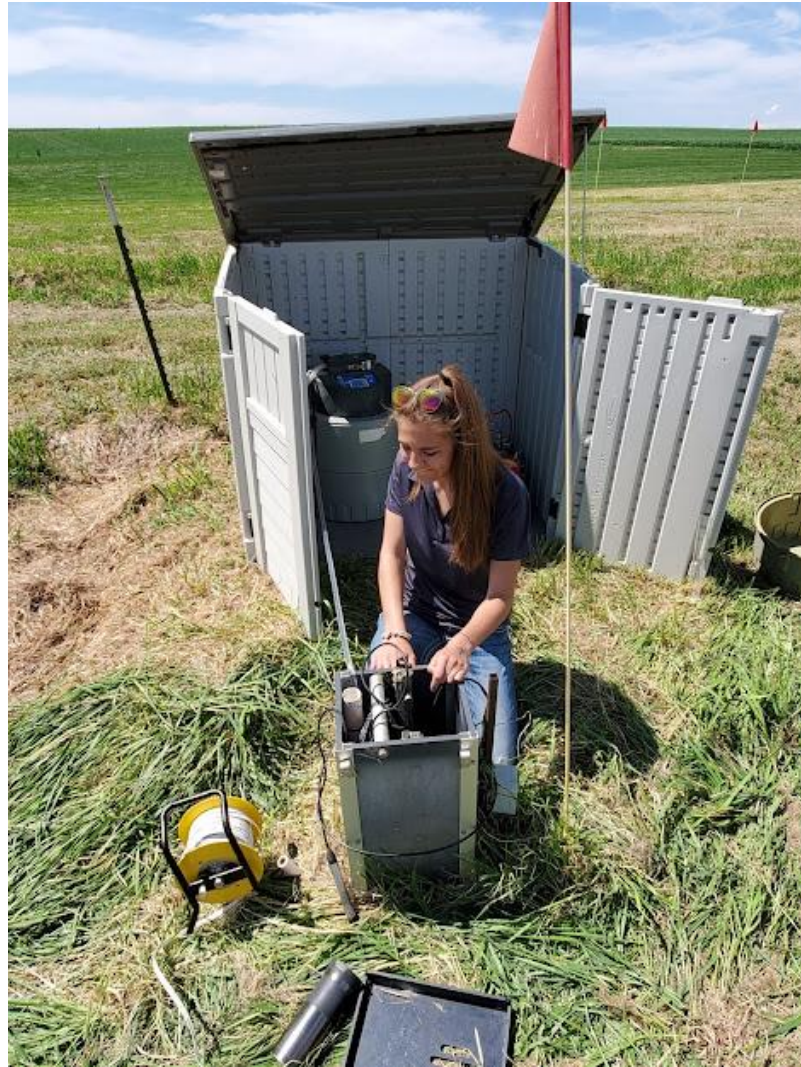
Figure 16: Outlet sampling station for tracer study at the Baltic, SD bioreactor
