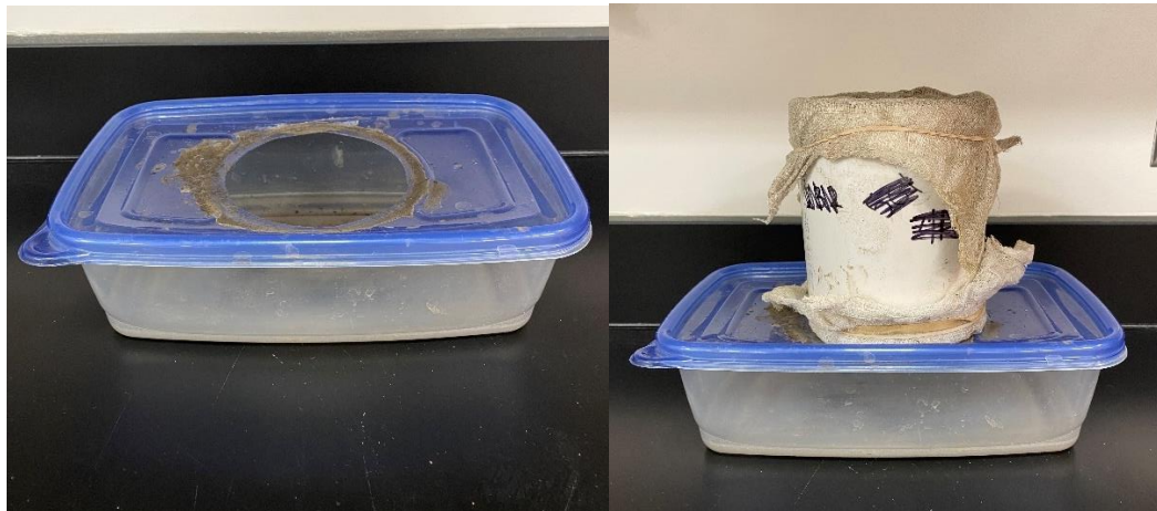
Figure 5: Photos of suspension system used to drain woodchip samples
