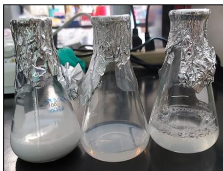
Figure 4.2 Emulsion visual stability test after 24 hours of mixed showing three different concentrations of oil-water used to stabilize the emulsion. From left to right: 4, 8, and 12 % of the surfactant Tween -80.
