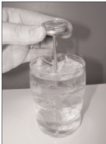
Insert thermometer into ice water without touching sides and bottom of glass.
